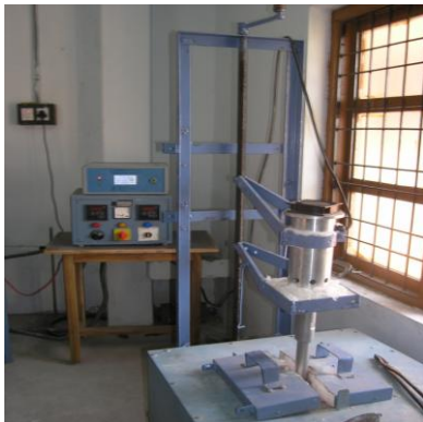
Fig 7: Experimental set up with Electrical Furnace, ultrasonic probe & Transducer
