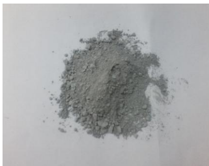
Fig 4: Alumina Powder after Ball milling of 30hrs
