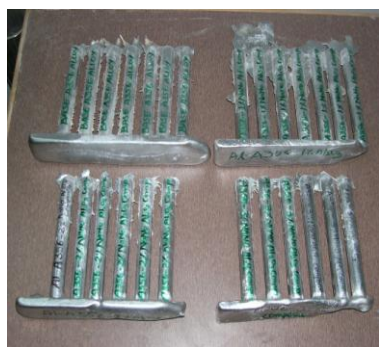
Fig 9: As cast cylindrical fingers of the A356- 0%, 1%, 2%, 3% nano alumina composite
