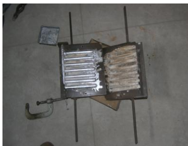
Fig 8: Metallic dies of Cylindrical finger casting
