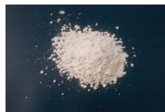
Fig 1: Pure Alumina ( Al_2O_3 ) Powder of 60 \mu m
